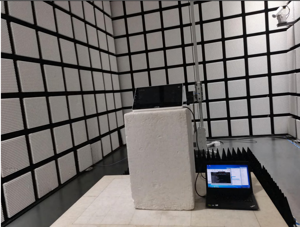
Fig. 3 Radiated emission setup photo(Above 1GHz)
