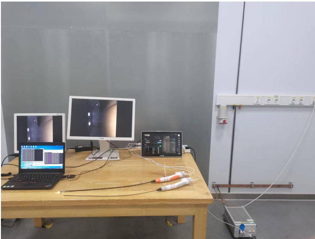
Fig. 4 Power line conducted emission setup photo
