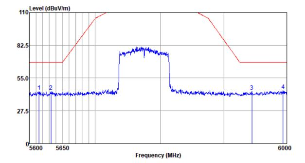
Mode:e; Polarization:Vertical; Modulation:c; bandwidth:80MHz; Channel:Low
