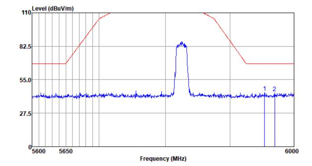
Mode:e; Polarization:Vertical; Modulation:a; bandwidth:20MHz; Channel:High
