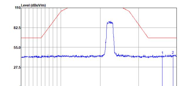
Mode:e; Polarization:Horizontal; Modulation:a; bandwidth:20MHz; Channel:High
