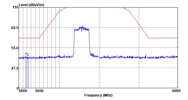
Mode:e; Polarization:Vertical; Modulation:n; bandwidth:40MHz; Channel:Low
