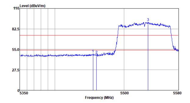
Mode:d; Polarization:Horizontal; Modulation:c; bandwidth:80MHz; Channel:Low
