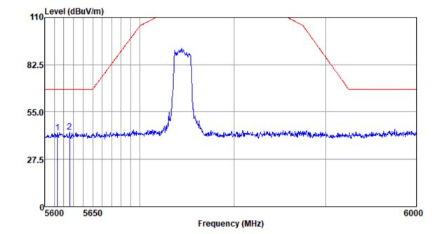
Mode:e; Polarization:Horizontal; Modulation:n; bandwidth:20MHz; Channel:Low
