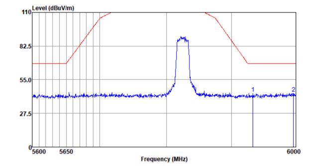
Mode:e; Polarization:Horizontal; Modulation:n; bandwidth:20MHz; Channel:High
