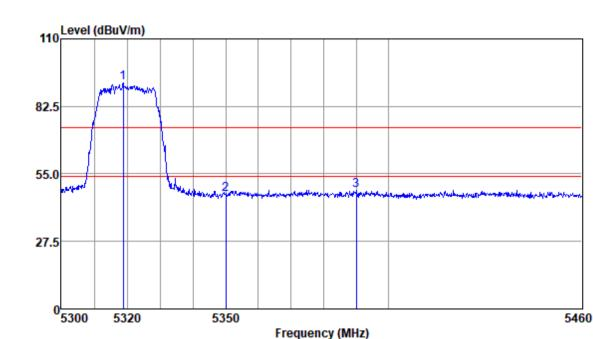
Mode:c; Polarization:Vertical; Modulation:c; bandwidth:20MHz; Channel:High
