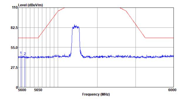
Mode:e; Polarization:Vertical; Modulation:n; bandwidth:20MHz; Channel:Low
