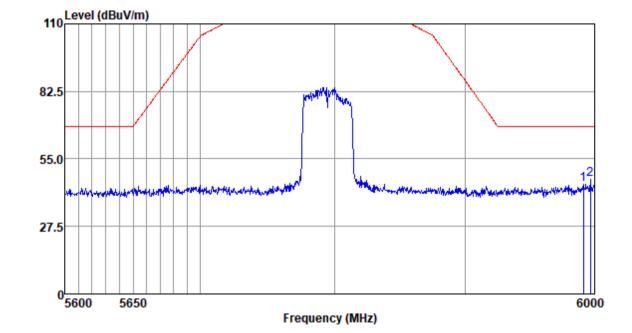
Mode:e; Polarization:Vertical; Modulation:n; bandwidth:40MHz; Channel:High
