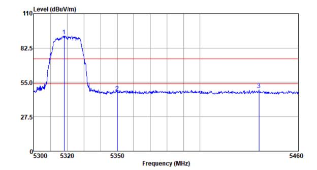
Mode:c; Polarization:Vertical; Modulation:a; bandwidth:20MHz; Channel:High
