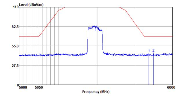
Mode:e; Polarization:Vertical; Modulation:c; bandwidth:40MHz; Channel:High
