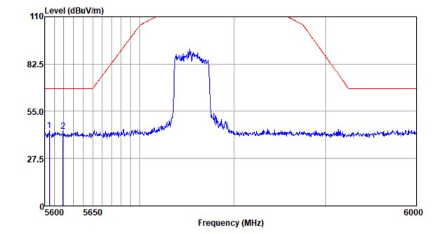
Mode:e; Polarization:Horizontal; Modulation:n; bandwidth:40MHz; Channel:Low
