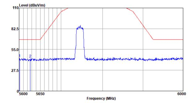
Mode:e; Polarization:Vertical; Modulation:a; bandwidth:20MHz; Channel:Low
