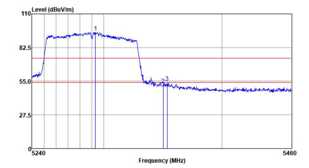
Mode:c; Polarization:Horizontal; Modulation:c; bandwidth:80MHz; Channel:High
