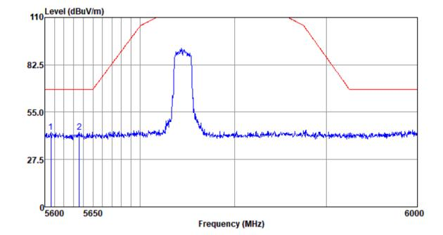
Mode:e; Polarization:Horizontal; Modulation:c; bandwidth:20MHz; Channel:Low
