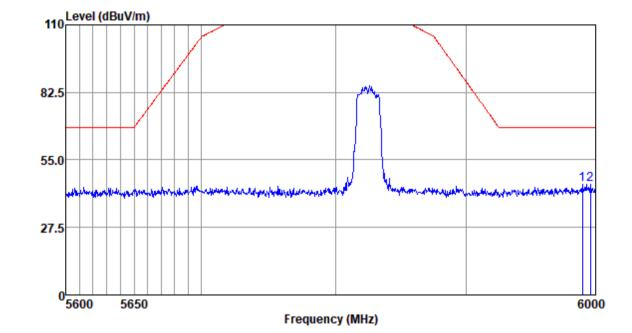
Mode:e; Polarization:Vertical; Modulation:n; bandwidth:20MHz; Channel:High
