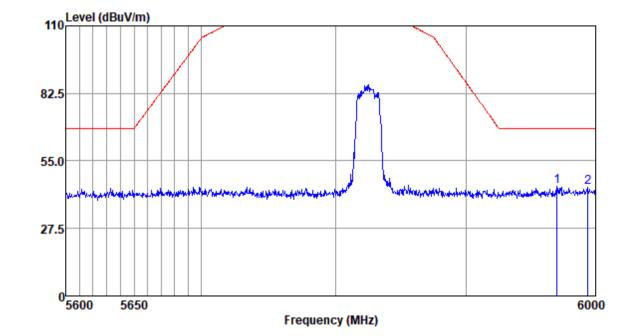
Mode:e; Polarization:Vertical; Modulation:c; bandwidth:20MHz; Channel:High
