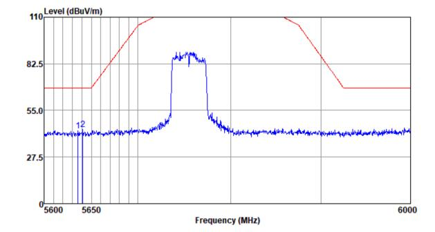
Mode:e; Polarization:Horizontal; Modulation:c; bandwidth:40MHz; Channel:Low
