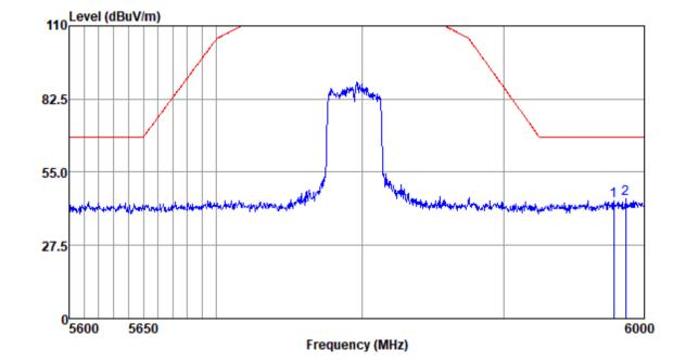
Mode:e; Polarization:Horizontal; Modulation:n; bandwidth:40MHz; Channel:High
