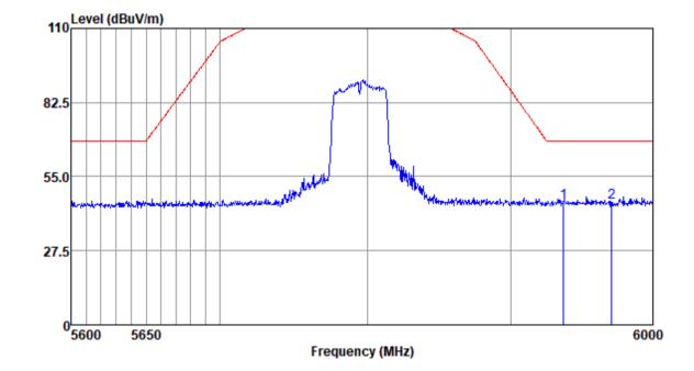
Mode:e; Polarization:Vertical; Modulation:n; bandwidth:40MHz; Channel:High
