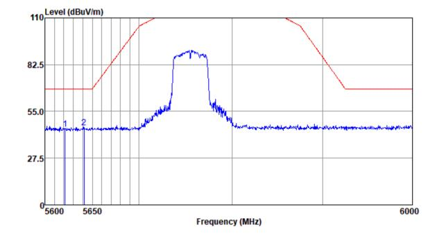
Mode:e; Polarization:Vertical; Modulation:n; bandwidth:40MHz; Channel:Low
