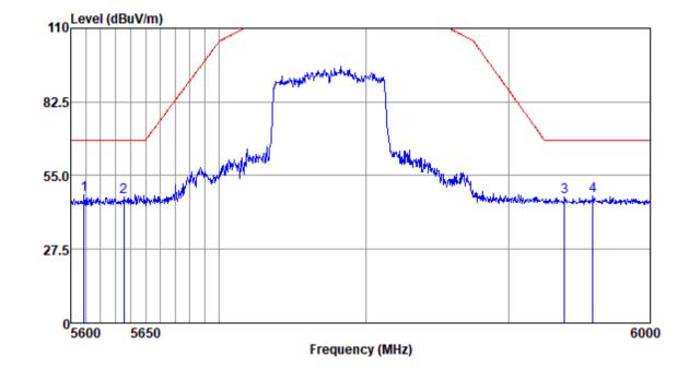
Mode:e; Polarization:Horizontal; Modulation:c; bandwidth:80MHz; Channel:Low
