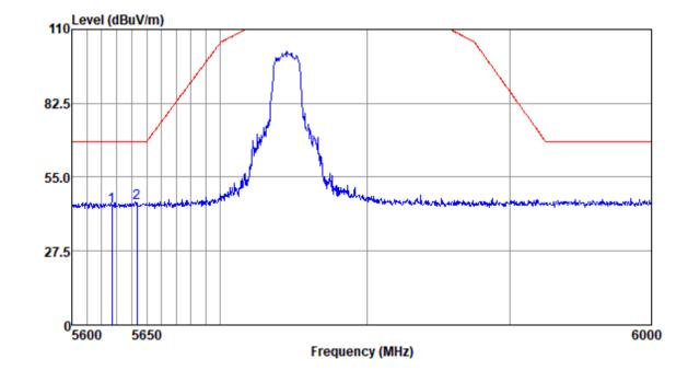
Mode:e; Polarization:Horizontal; Modulation:c; bandwidth:20MHz; Channel:Low
