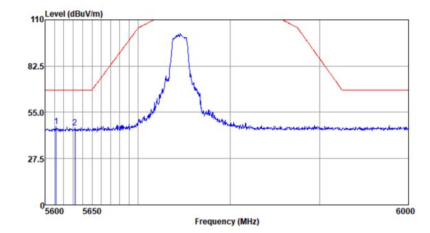
Mode:e; Polarization:Horizontal; Modulation:a; bandwidth:20MHz; Channel:Low
