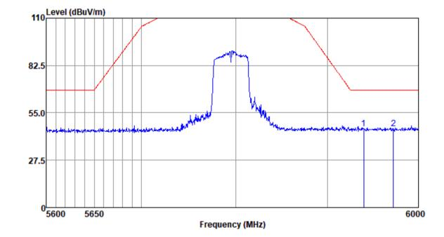
Mode:e; Polarization:Vertical; Modulation:c; bandwidth:40MHz; Channel:High
