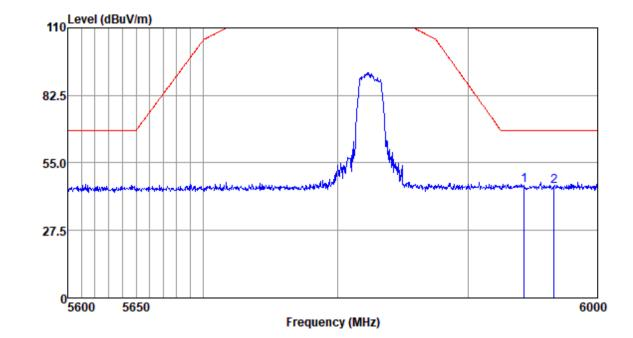
Mode:e; Polarization:Vertical; Modulation:n; bandwidth:20MHz; Channel:High
