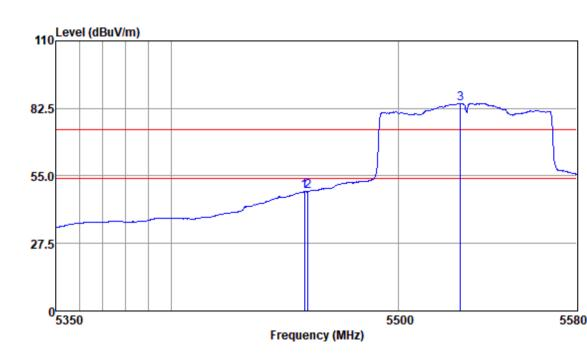
Mode:d; Polarization:Horizontal; Modulation:c; bandwidth:80MHz; Channel:Low
