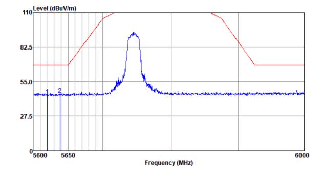
Mode:e; Polarization:Vertical; Modulation:a; bandwidth:20MHz; Channel:Low
