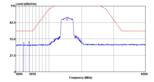
Mode:e; Polarization:Vertical; Modulation:c; bandwidth:40MHz; Channel:Low
