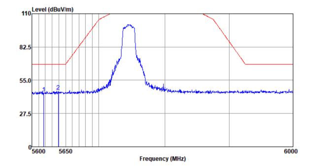
Mode:e; Polarization:Horizontal; Modulation:n; bandwidth:20MHz; Channel:Low
