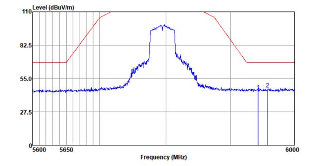
Mode:e; Polarization:Horizontal; Modulation:c; bandwidth:40MHz; Channel:High
