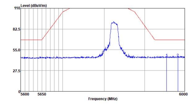
Mode:e; Polarization:Vertical; Modulation:a; bandwidth:20MHz; Channel:High
