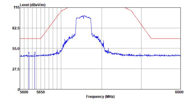
Mode:e; Polarization:Horizontal; Modulation:c; bandwidth:40MHz; Channel:Low
