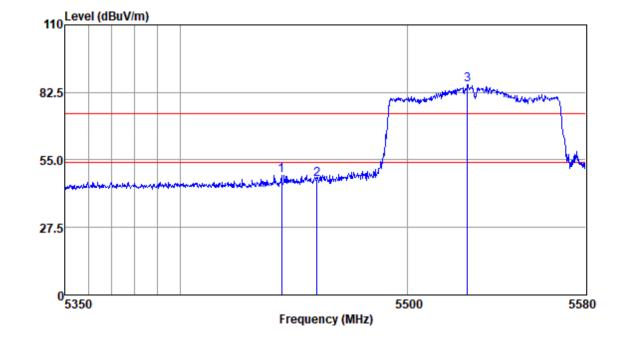
Mode:d; Polarization:Vertical; Modulation:c; bandwidth:80MHz; Channel:Low
