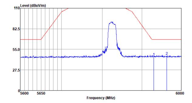
Mode:e; Polarization:Vertical; Modulation:c; bandwidth:20MHz; Channel:High
