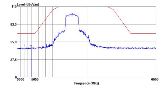
Mode:e; Polarization:Horizontal; Modulation:n; bandwidth:40MHz; Channel:Low
