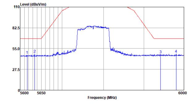
Mode:e; Polarization:Vertical; Modulation:c; bandwidth:80MHz; Channel:Low
