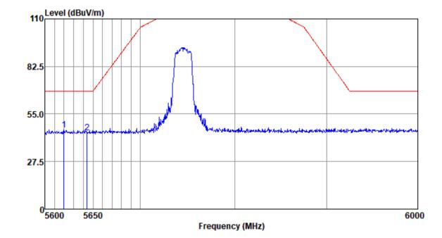
Mode:e; Polarization:Vertical; Modulation:n; bandwidth:20MHz; Channel:Low
