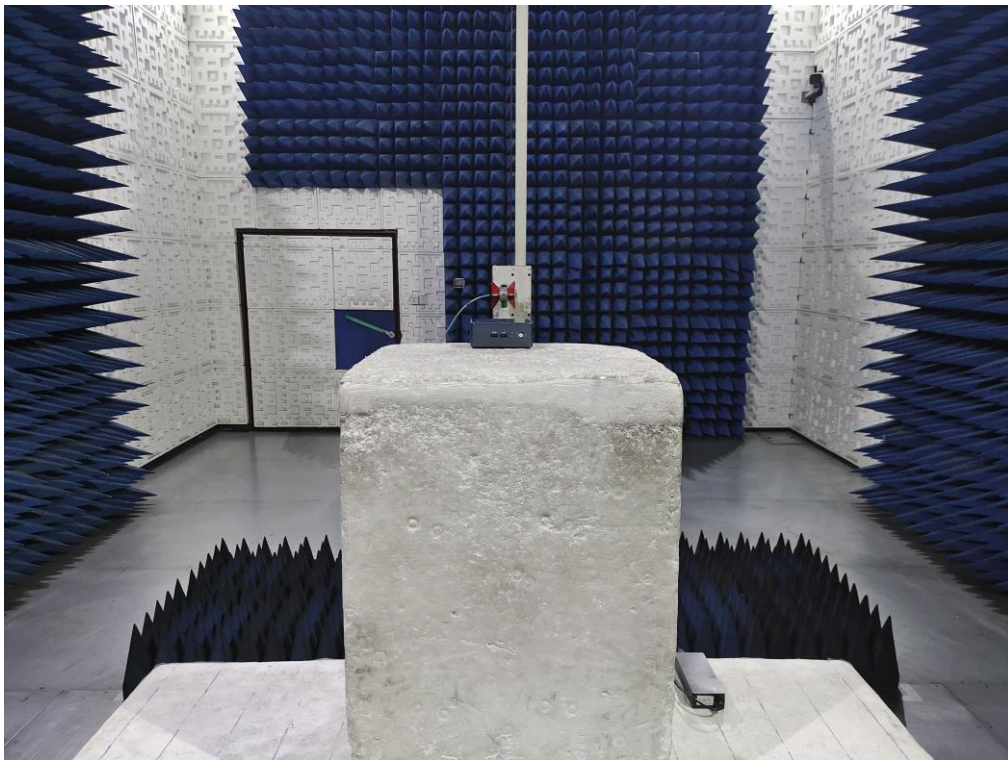
RADIATED EMISSION TEST SETUP ABOVE 1GHz
