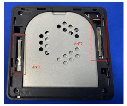
The antenna is metal antenna. Ant 1: 2.48dBi; Ant2: 1.94dBi (provided by the applicant)
