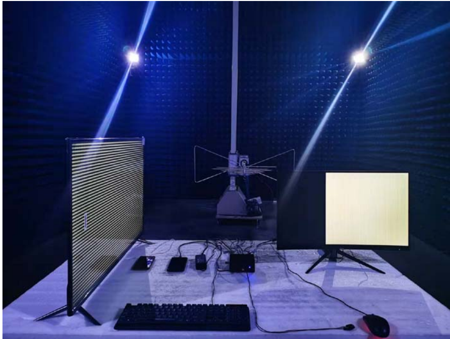
Photo of Radiated Emission Measurement (Below 1G)
