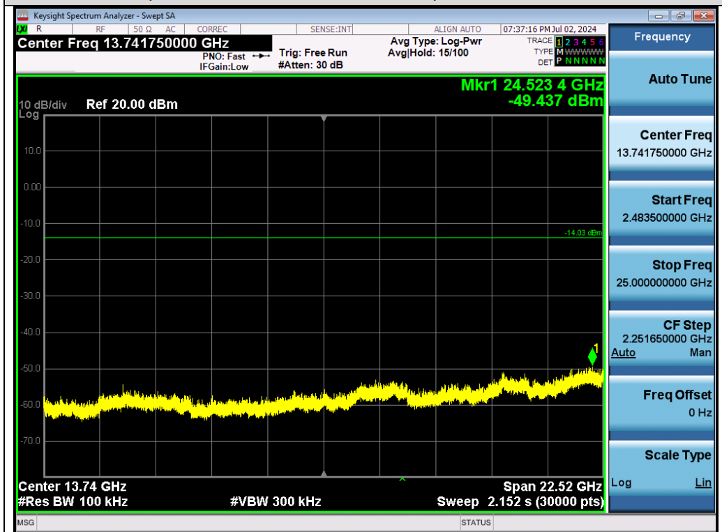
Test_Graph_802.11b_Chain A_2412_1Mbps_Higher Band Emissions
