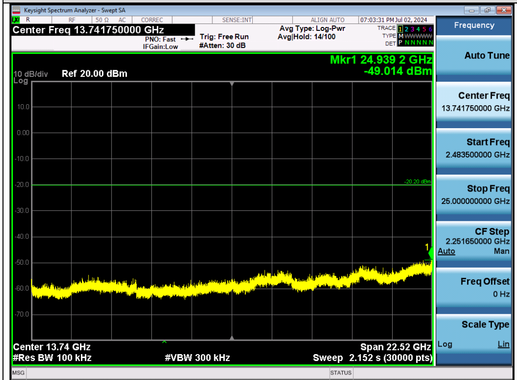
Test_Graph_802.11n40_Chain B_2422_MCS0_Higher Band Emissions
