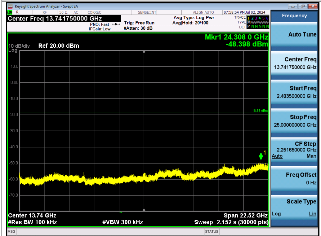
Test_Graph_802.11n20_Chain A_2412_MCS0_Higher Band Emissions
