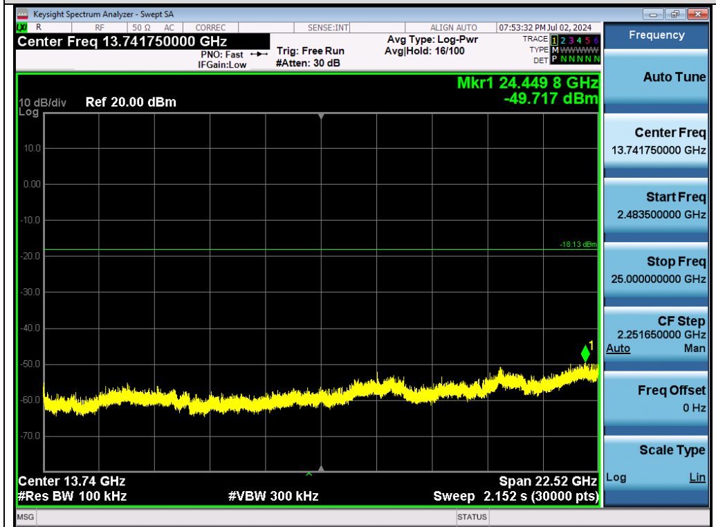
Test_Graph_802.11g_Chain A_2437_6Mbps_Higher Band Emissions
