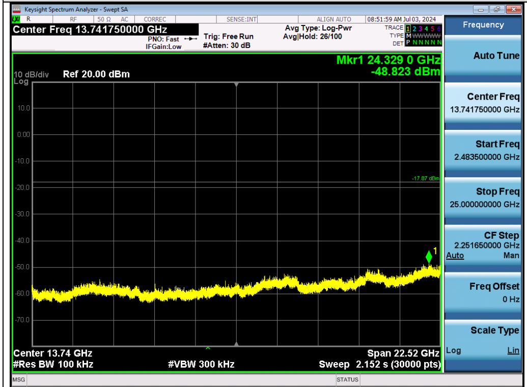
Test_Graph_802.11ax20_Chain A_2412_MCS0_Higher Band Emissions
