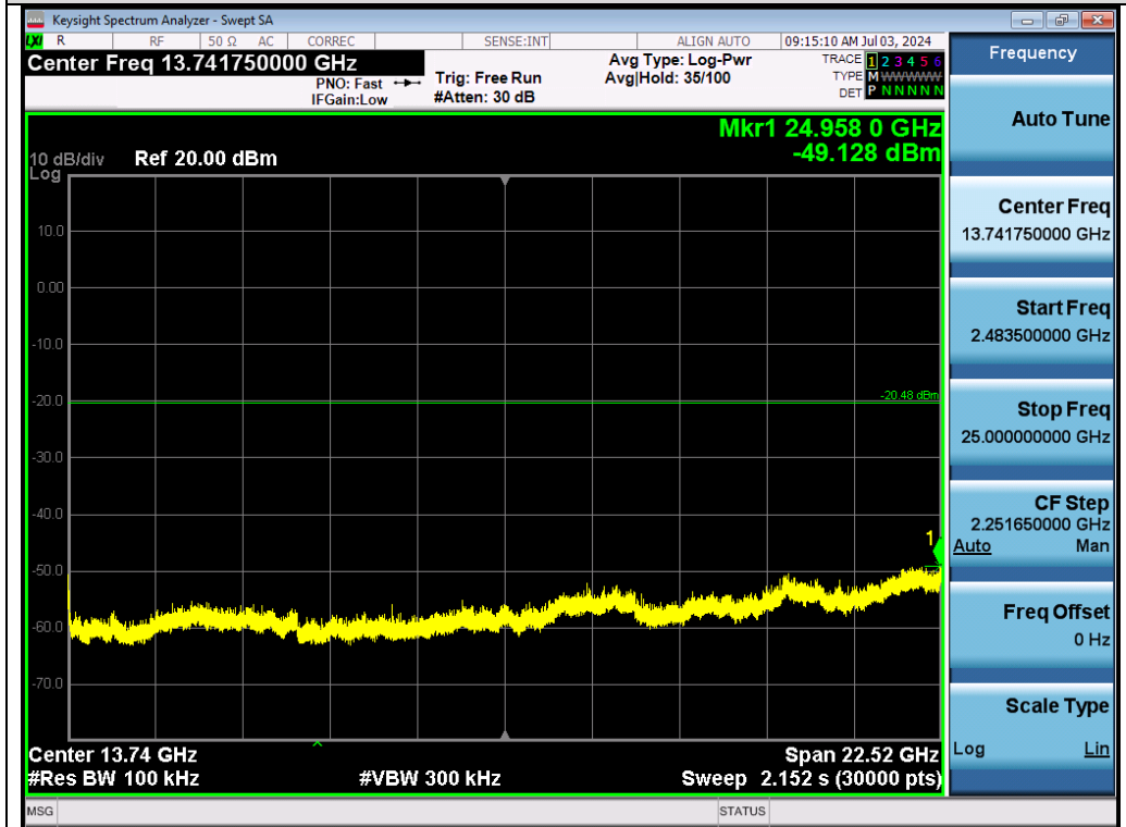
Test_Graph_802.11ax40_Chain A_2437_MCS0_Higher Band Emissions
