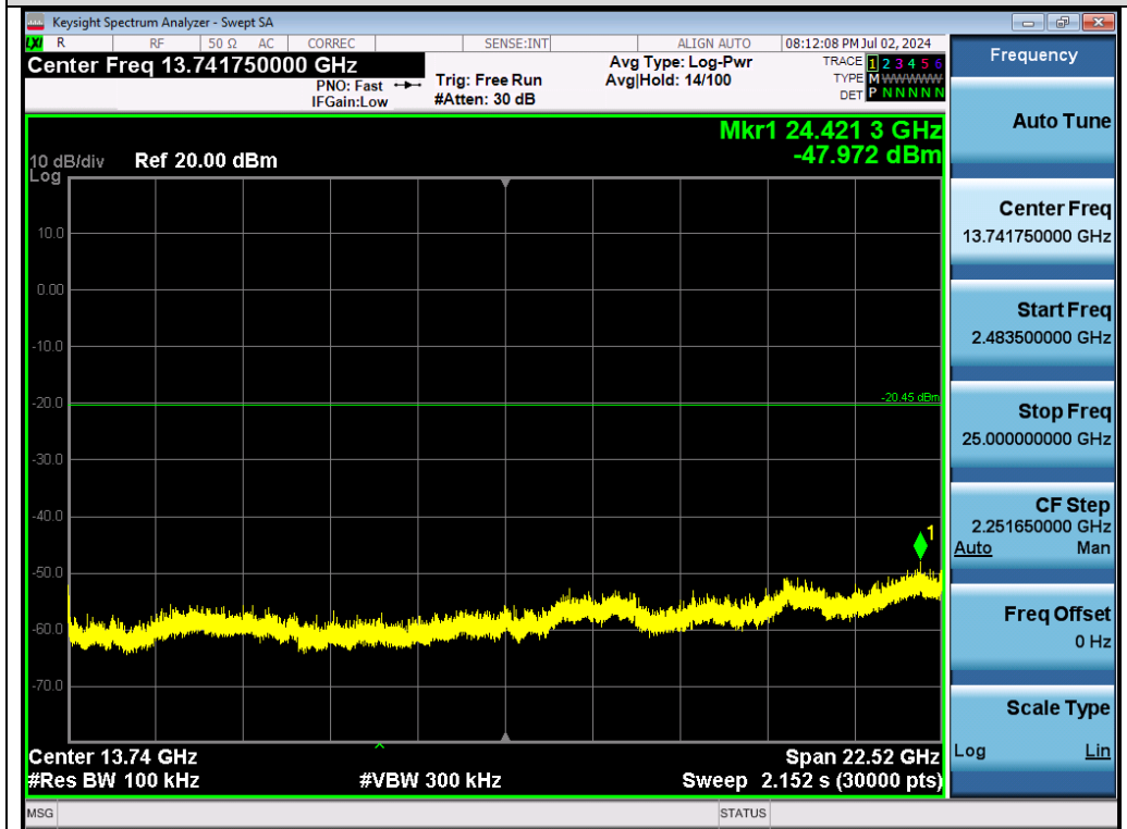
Test_Graph_802.11n40_Chain A_2437_MCS0_Higher Band Emissions
