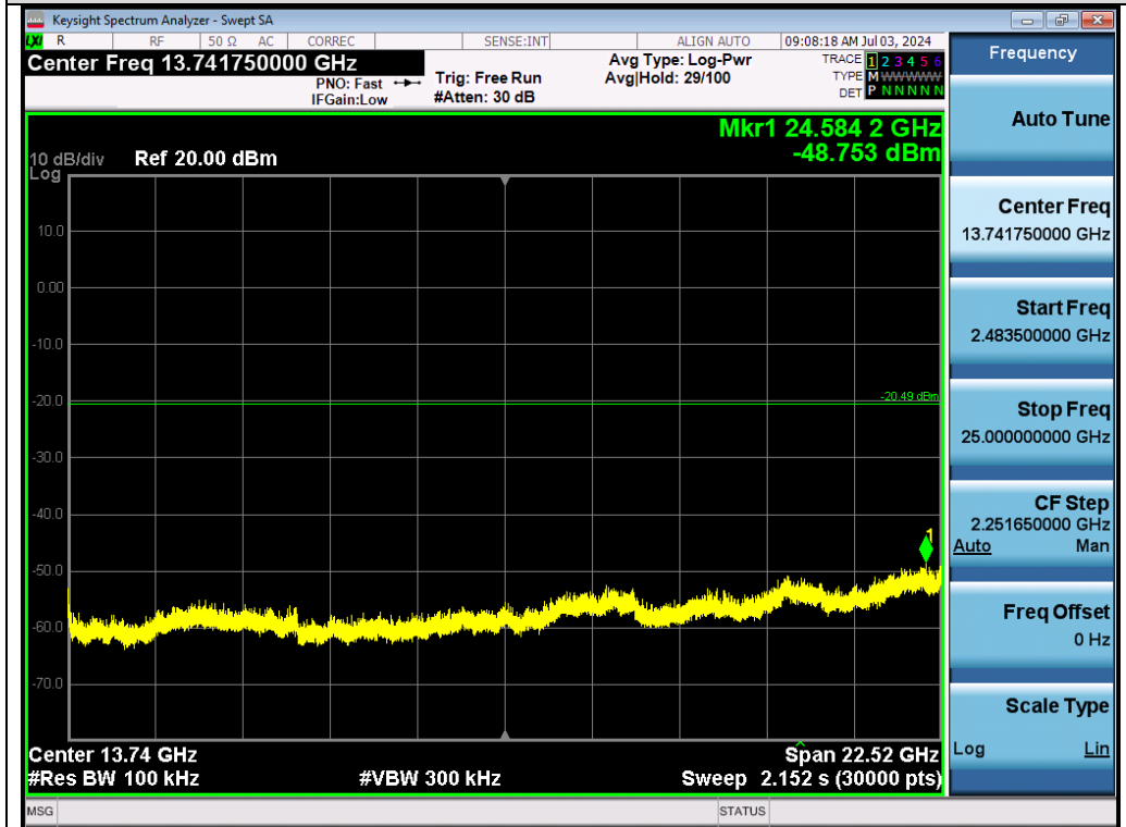
Test_Graph_802.11ax40_Chain A_2422_MCS0_Higher Band Emissions
