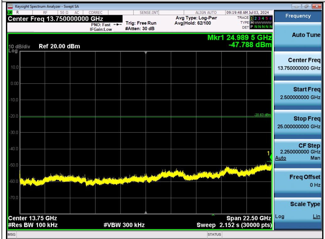
Test_Graph_802.11ax40_Chain A_2452_MCS0_Higher Band Emissions
