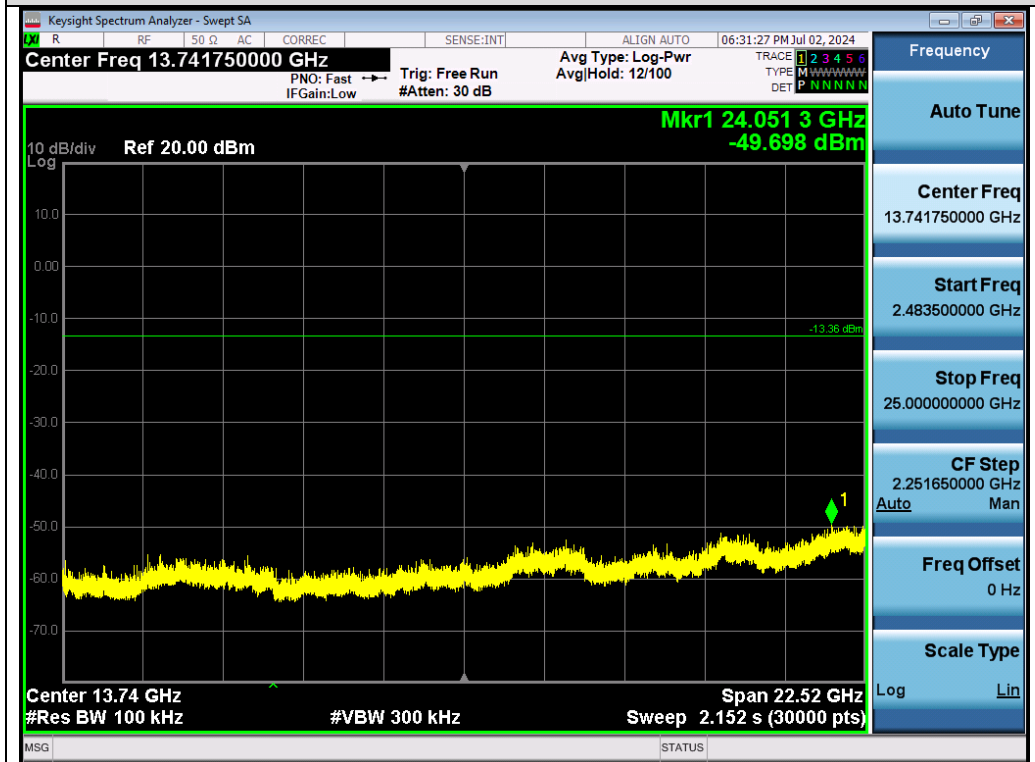
Test_Graph_802.11b_Chain B_2437_1Mbps_Higher Band Emissions
