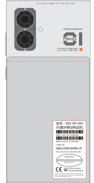
The label will be attached to the product using special glue, the label drawing isn't removed easily.
