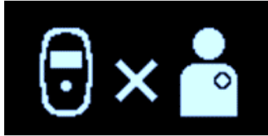
Figure 56: Charger/IPG Pairing Error Screen
