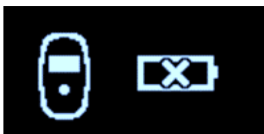
Figure 67: Low Charger Battery Alert Screen
