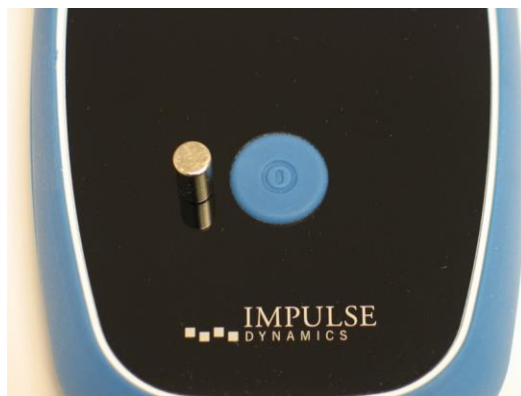
Figure 76: Pairing Magnet on Vesta Charger
