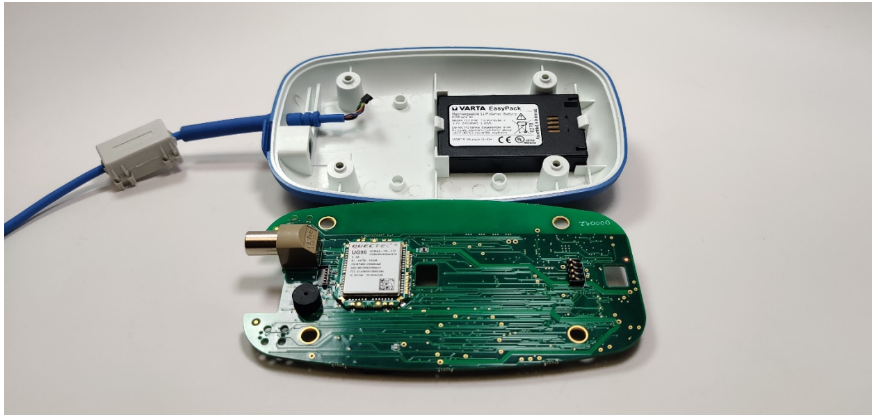
Internal Picture 6: Bottom PCB layout after removal from battery/enclosure and connector to charging coil board.
