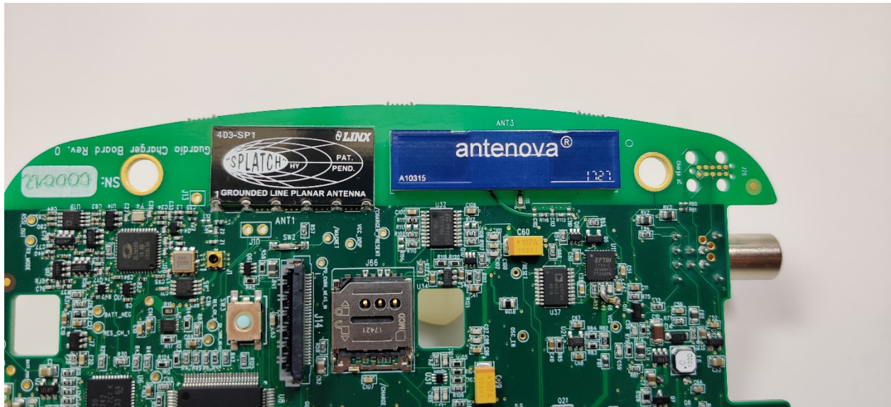
Internal Picture 3: Antennas present on the main board. 403MHz MICs antenna is Linx Technologies ANT-403-SP (left, black). GSM/UMTS antenna is Antenova A10315 that is disabled in Vesta Charger systems (right, blue).
