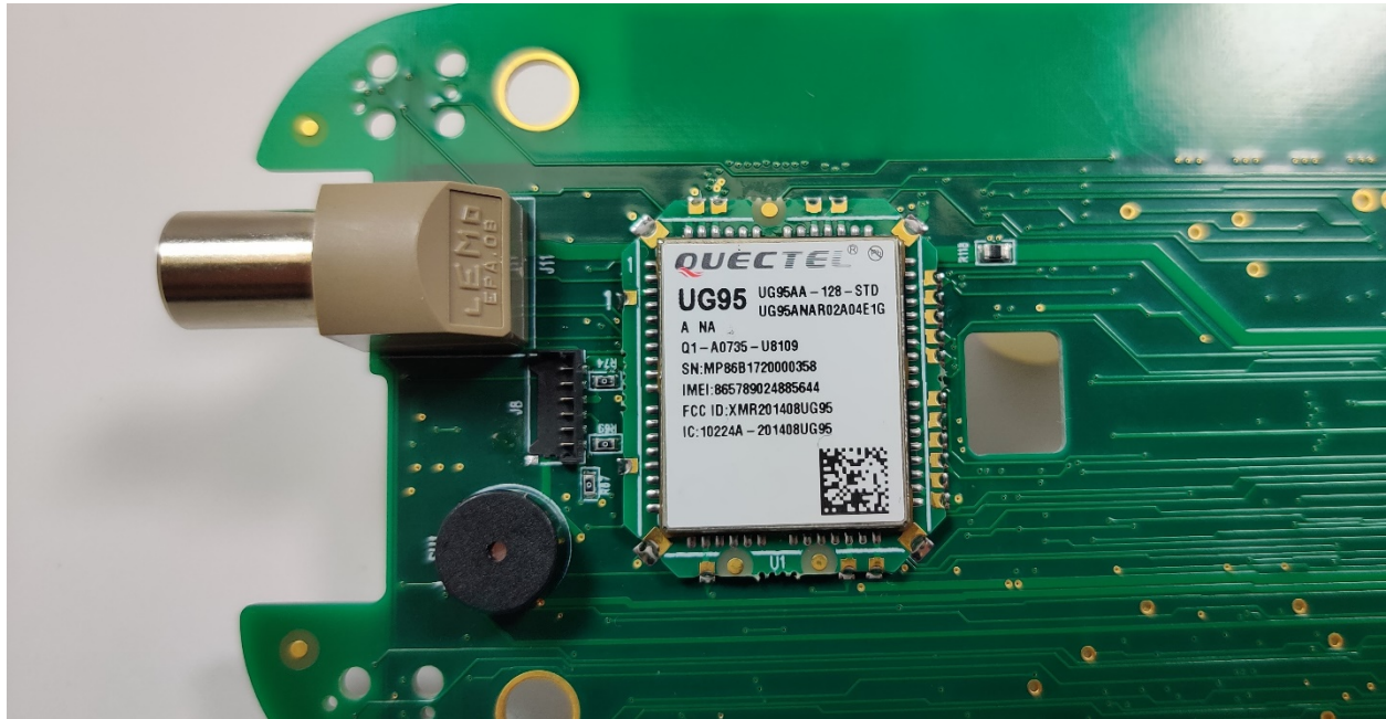
Internal Picture 5: Quetel UG95 3G modem that is firmware disabled in the Vesta Charger systems, but is populated.
