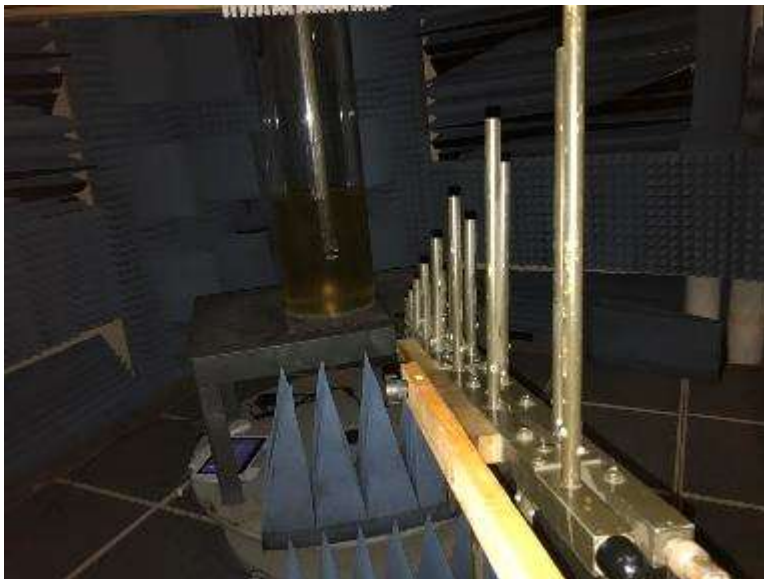
EUT Inside Torso Simulator for Loss Measurement
