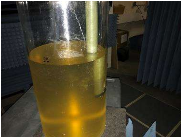
Side View of EUT in Torso Simulator
