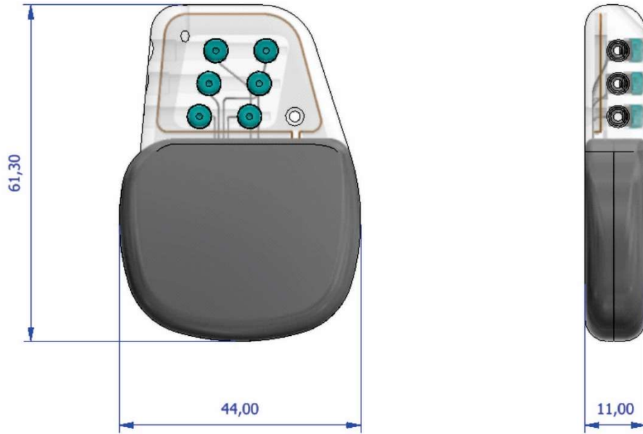
External Picture 2: Computer generated model showing dimensions and volume of implant. Dimensional units are in millimeters, and volume units are in cubic centimeters.
