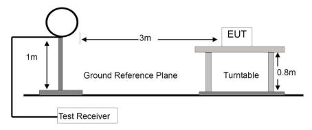
For Radiated Emission 30-1000MHz
