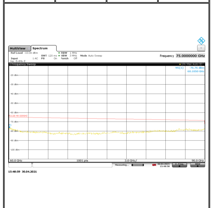
Plot# 61 Radiated Emission 60-90GHz
