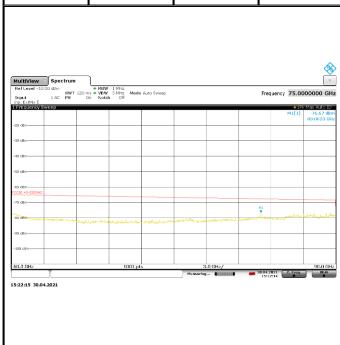
Plot# 38 Radiated Emission 60-90GHz
