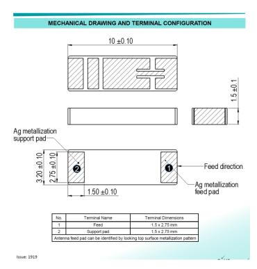
**FCC 15.203 Compliance:** Antenna is a surface mount ceramic chip package soldered directly to the PCB. Antenna is not a user serviceable part.
