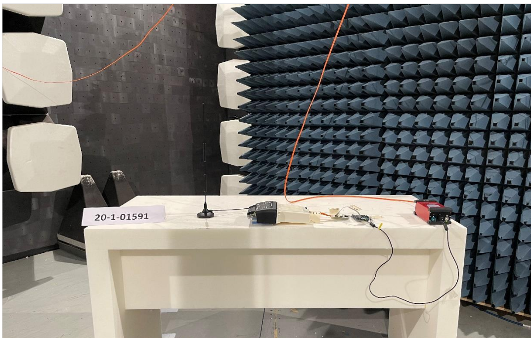
Photograph 2: EUT Test Setup in the semi anechoic chamber, Radiated interference field strength
