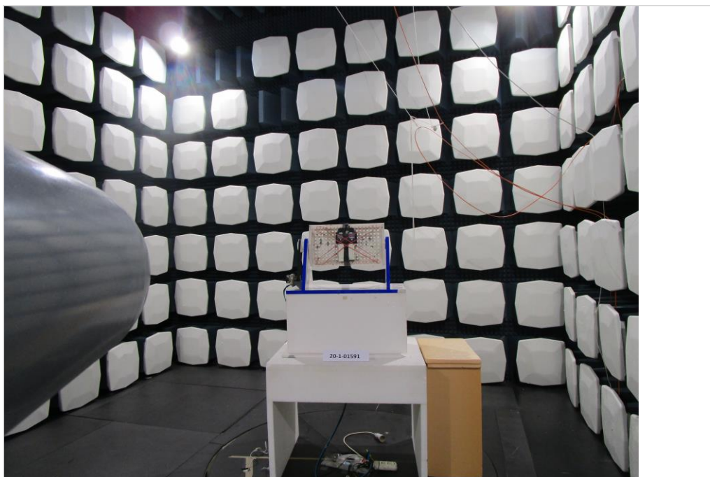
Photograph 4: EUT Test Setup in the fully anechoic chamber, overall view
