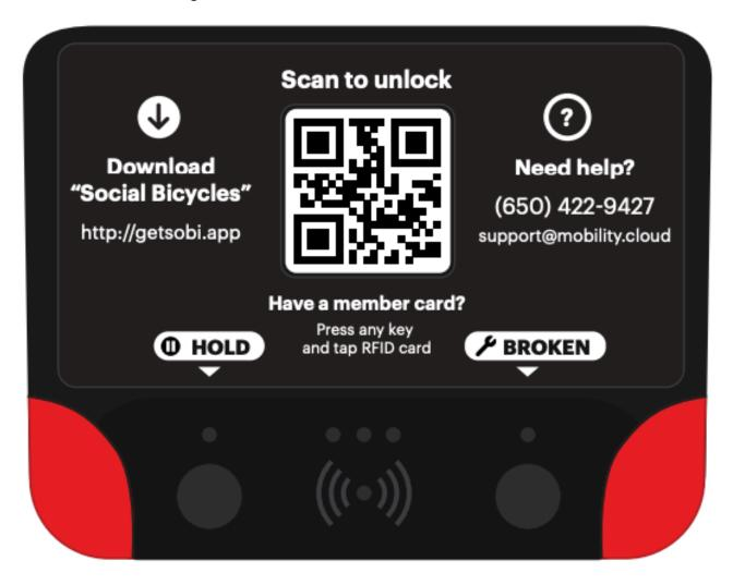
The two large circles are capacitive touch buttons intended for users to interact with the device. The left button puts a ride on hold, the right button reports issues with the bike, and all buttons wake up the module. The three small LEDs in the middle are use for status indication of the bicycle. The area in the middle is where the RFID antenna is located, and allows to start rental using RFID card.
