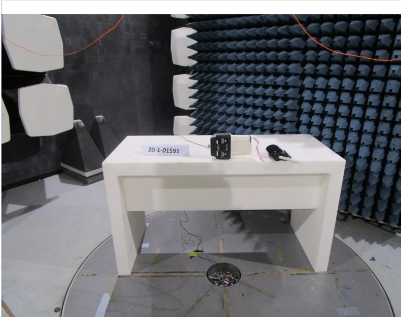
Photograph 1: EUT test setup in the semi anechoic chamber, close up view
