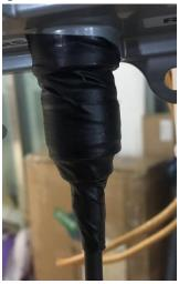
Cut a piece of waterproof glue, stretch it and wrap it along the RF port
