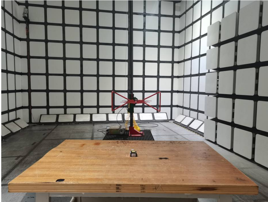
Radiated Emissions View (Below 1 GHz)
