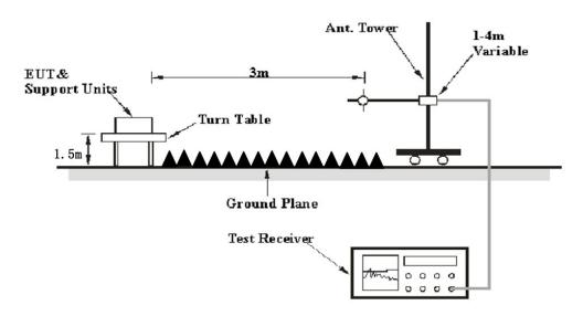
The radiated emission and out of band emission tests were performed in the 3 meters chamber test site, using the setup accordance with the ANSI C63.10-2013. The specification used was the FCC 15.209/15.205 and FCC 15.249 limits.
