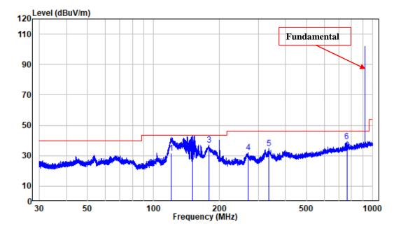
Site : chamber Condition: 3m VERTICAL Job No. : XMTN220217-04827E-RF Test Mode: 925 TX
