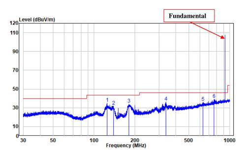
Site : chamber Condition: 3m HORIZONTAL Job No. : XMTN220217-04827E-RF Test Mode: 920 Transmitting
