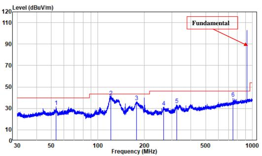
Site : chamber Condition: 3m VERTICAL Job No. : XMTN220217-04827E-RF Test Mode: 920 TX
