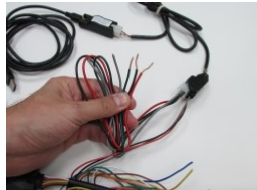
Use the red and black wires for the power supply (see section 5)
