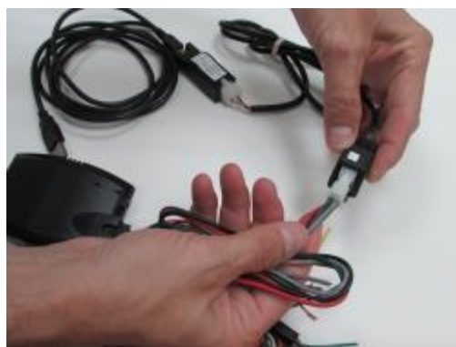
Connect one side of the power cable to the eNet hub
