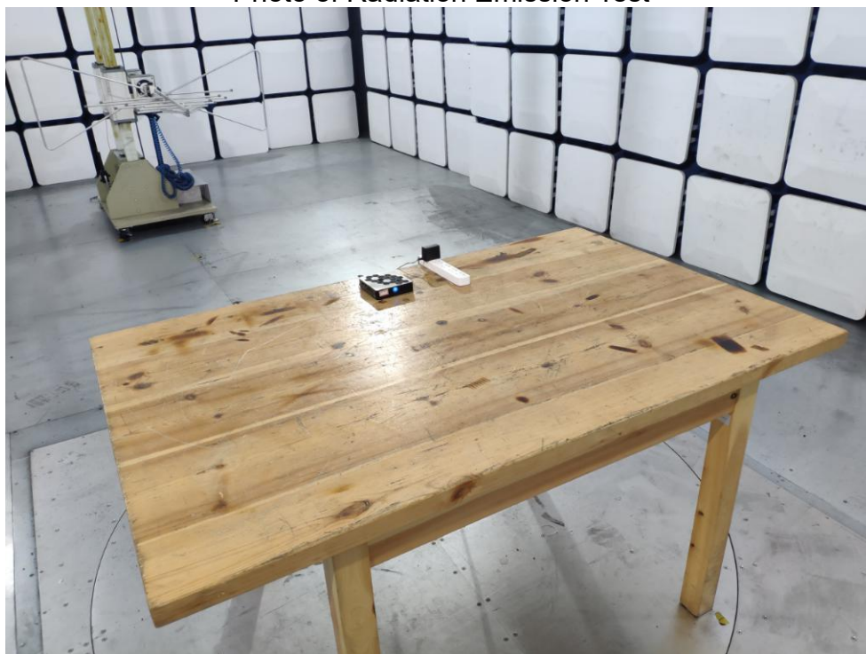
Photo of Radiation Emission Test
