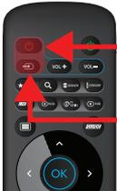
1. On the BT-250, press and hold the TV POWER + TV SOURCE for 3 seconds. Once the red light turns on, release the buttons.
