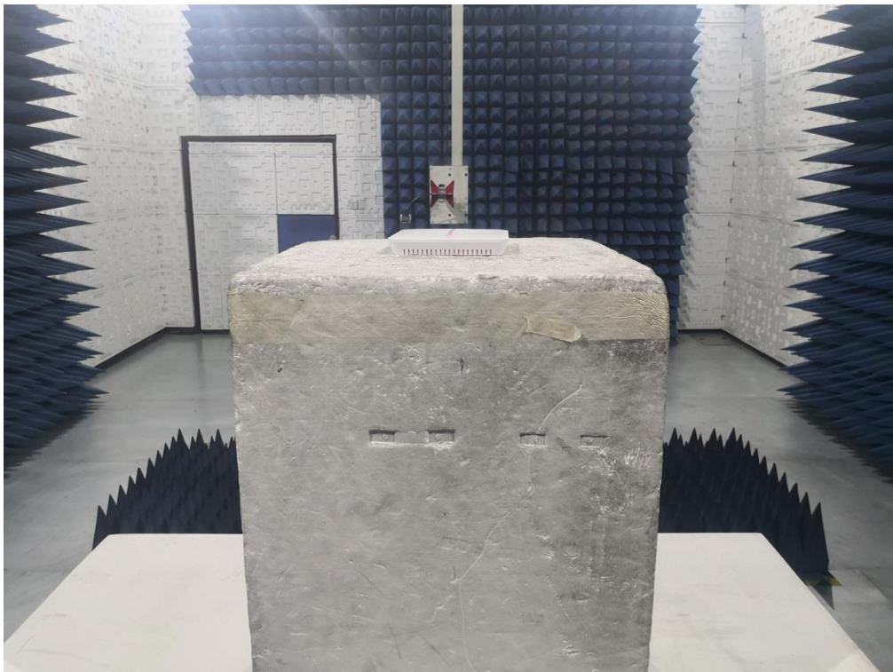
RADIATED EMISSION TEST SETUP ABOVE 1GHZ
