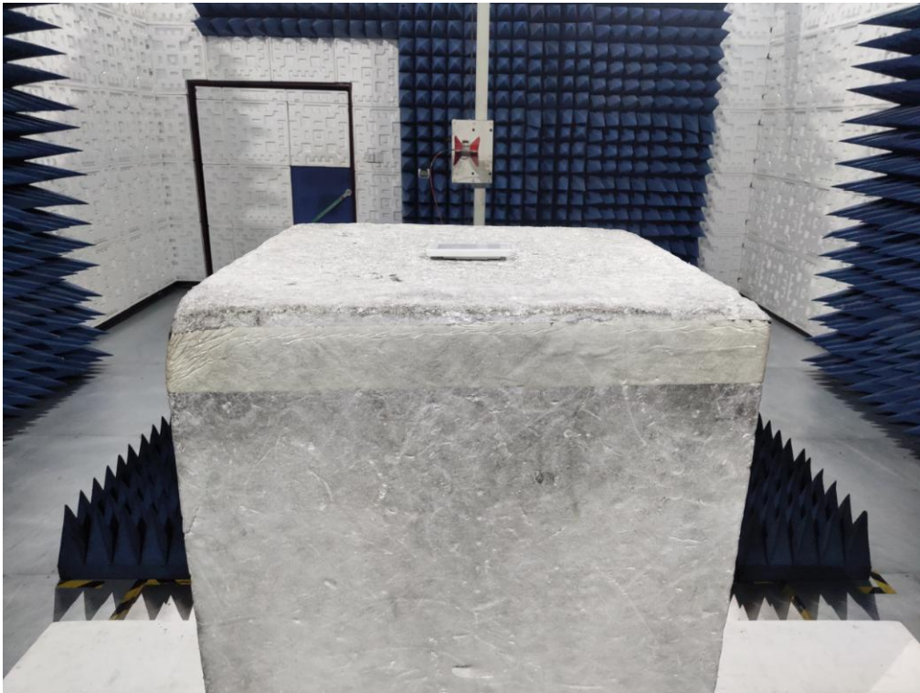
RADIATED EMISSION TEST SETUP ABOVE 1GHZ
