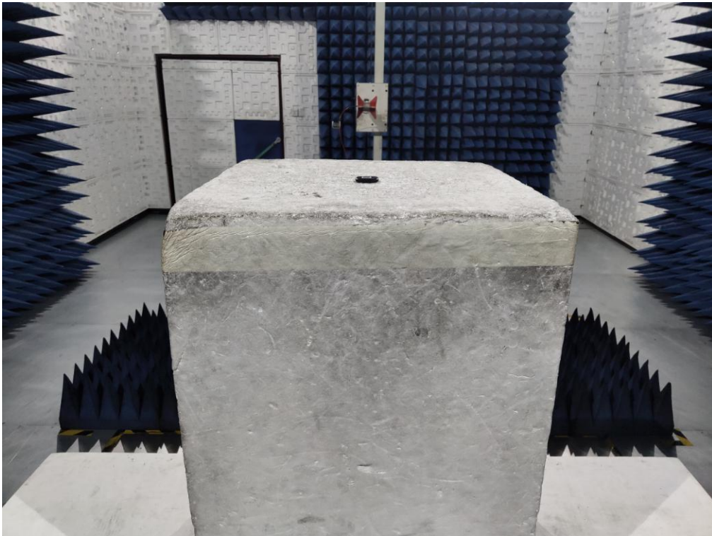
RADIATED EMISSION TEST SETUP ABOVE 1GHZ
