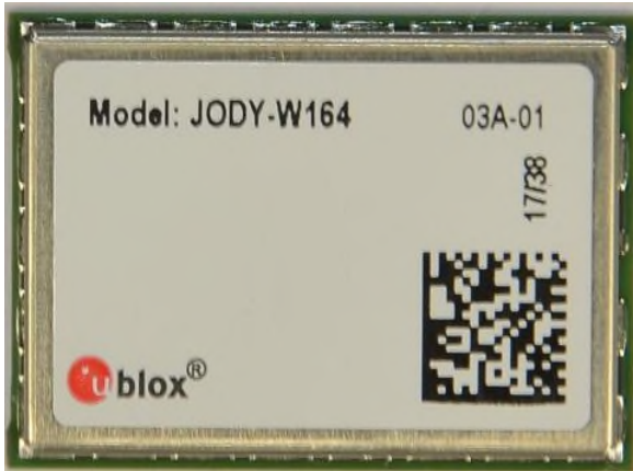
Figure 3: JODY-W164-03A top view external photo
