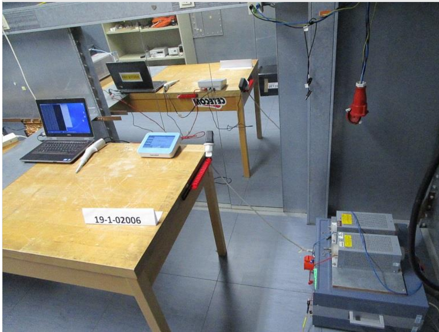
Photograph 1: EUT test setup Conducted emissions on AC-Power lines
