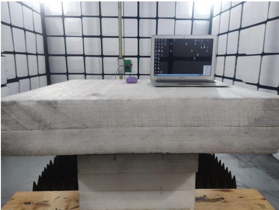
Photo of Radiation Emission Test
