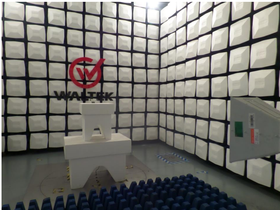
Test Setup For Radiated Emission (Above 1GHz)
