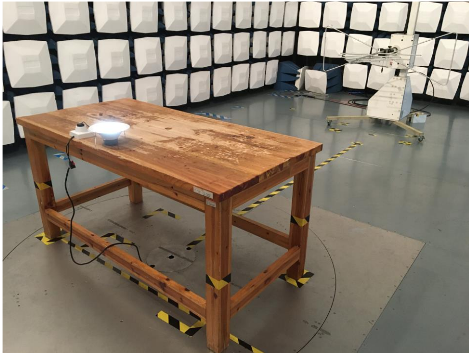
Test Setup For Radiated Emission (30MHz to 1GHz)
