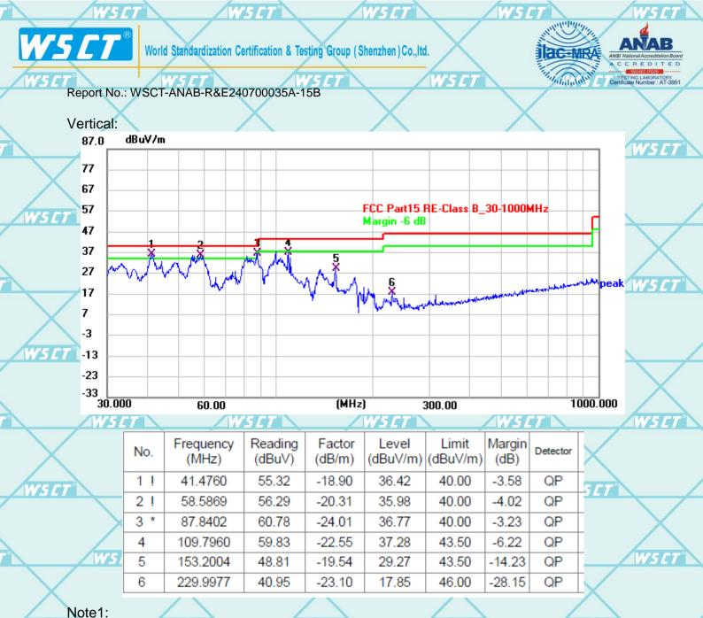
Freq. = Emission frequency in MHz WSC7 Reading level  $(dB\mu V)$  = Receiver reading Corr. Factor (dB) = Antenna factor + Cable loss - Amplifier factor. Measurement  $(dB\mu V)$  = Reading level  $(dB\mu V)$  + Corr. Factor (dB)Limit  $(dB\mu V)$  = Limit stated in standard Margin (dB) = Measurement  $(dB\mu V)$  – Limits  $(dB\mu V)$
