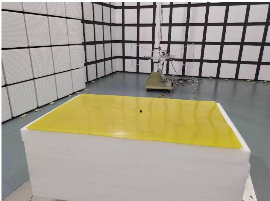
Photo of Radiated Emission Measurement (Below 1G)
