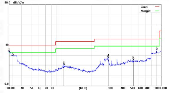
Polarization: Vertical / Band: 2.4G / BW: 1 / CH: H
