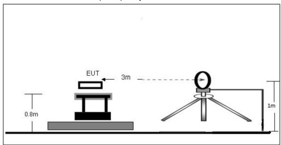
(B) Radiated Emission Test-Up Frequency 30MHz~1GHz
