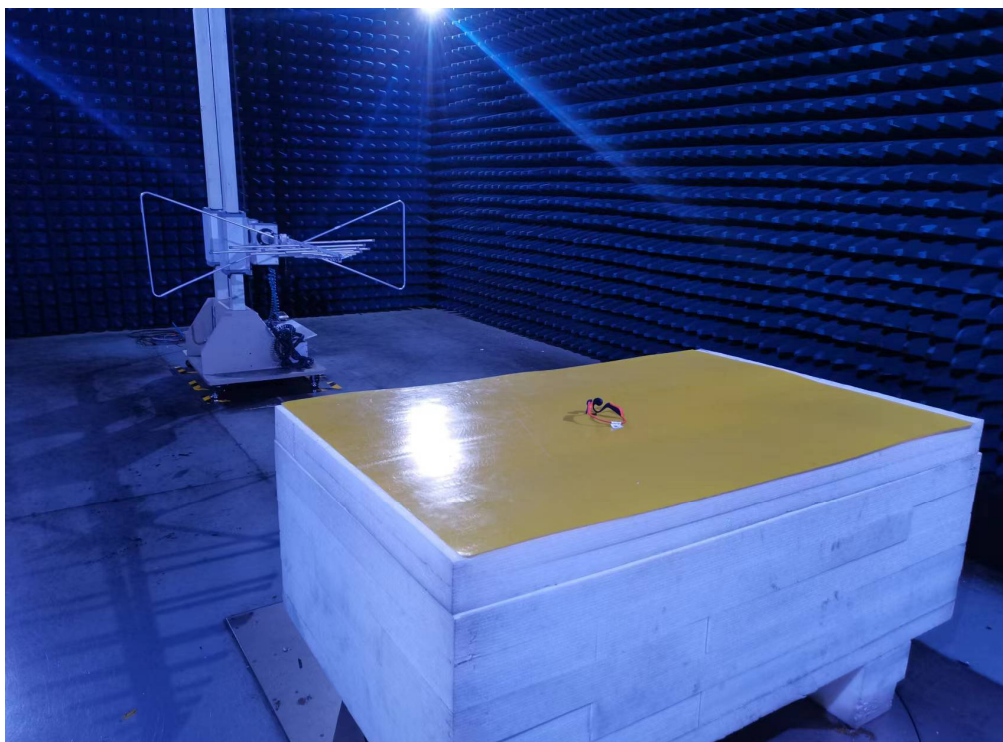
Photo of Radiated Emission Measurement (Above 1G)
