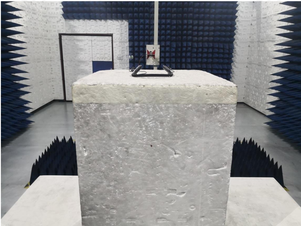
RADIATED EMISSION TEST SETUP ABOVE 1GHZ
