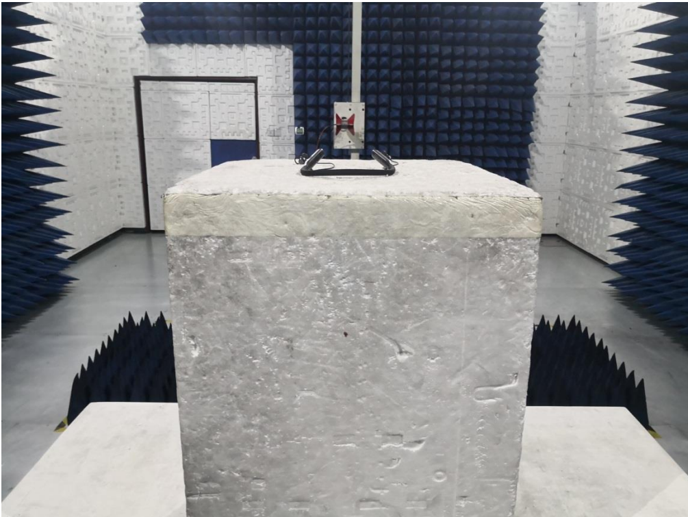
RADIATED EMISSION TEST SETUP ABOVE 1GHz
