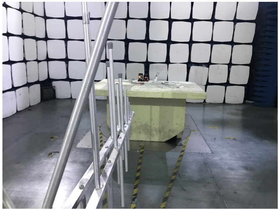
Radiation Emission Test Setup (30MHz to 1GHz)
