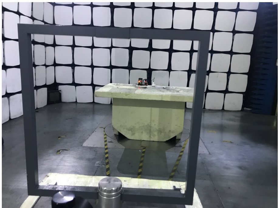
Radiation Emission Test Setup (Below 30MHz)
