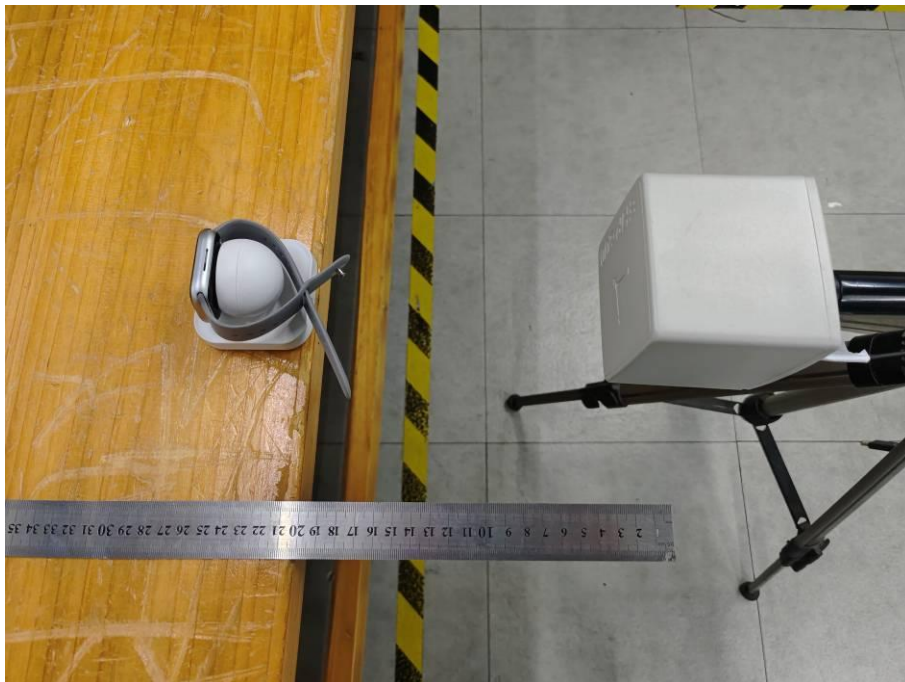
Test Position D-20cm from the edge of EUT to the geometric center of the probe
