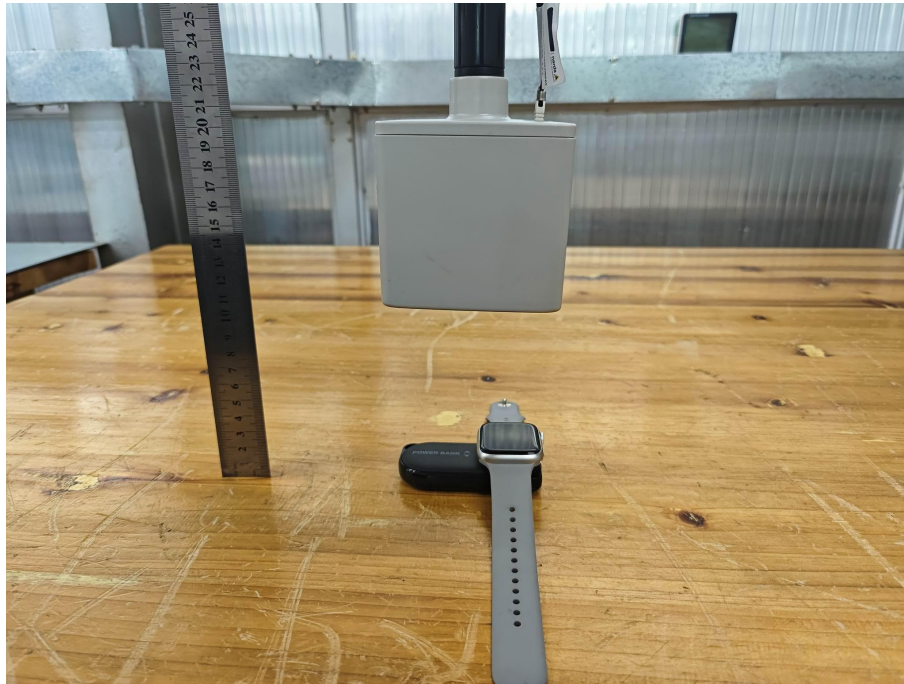
Test Position F-15cm from the edge of EUT to the geometric center of the probe
