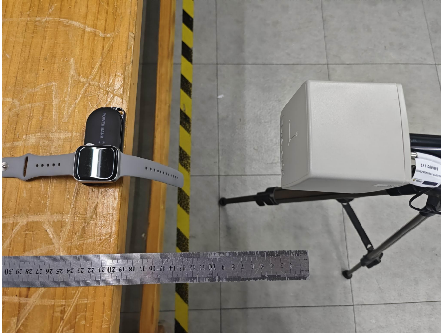
Test Position C-20cm from the edge of EUT to the geometric center of the probe
