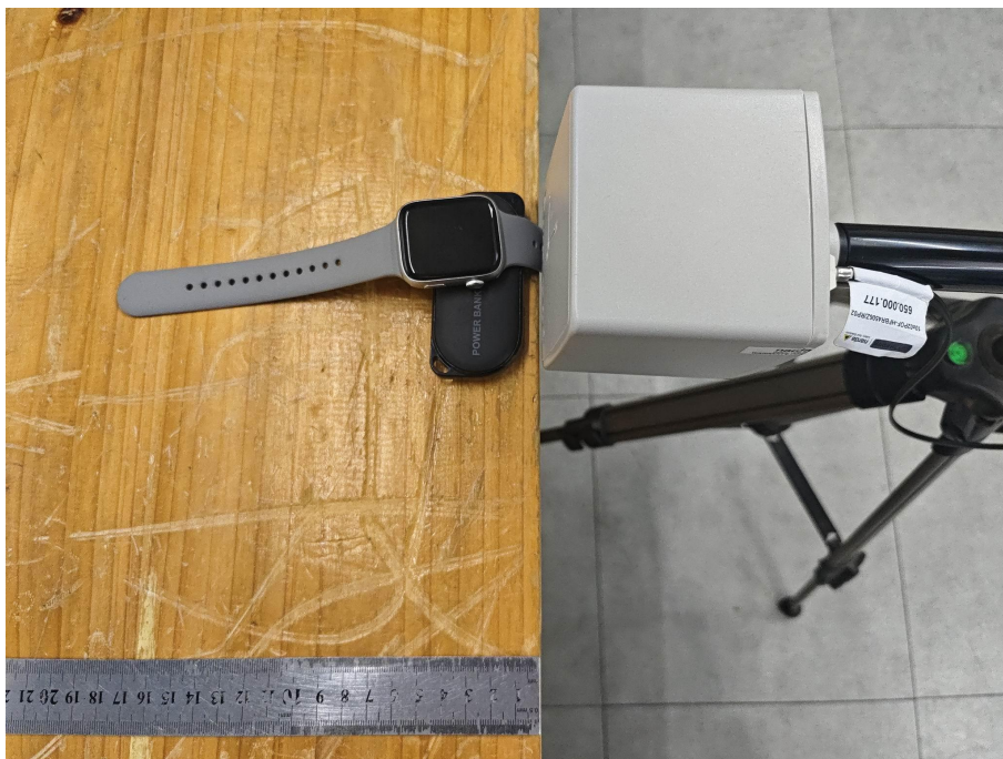
Test Position D-0cm from the edge of EUT to the geometric center of the probe
