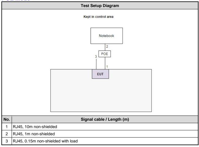
Note: The USB cable and fixture are disconnected from EUT and removed from test table when EUT is set to transmit continuously.
