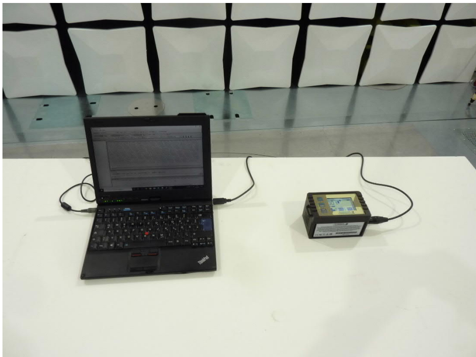
201626_10: EUT setup radiated emission data exchange mode
