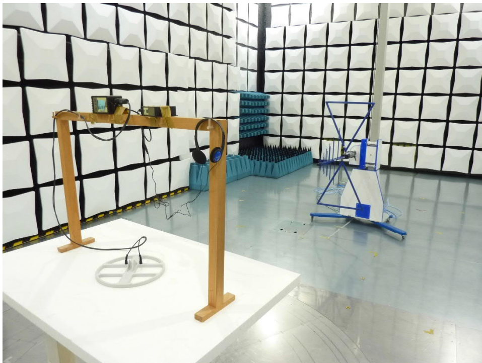
201626_04: EUT setup radiated emission 35 cm DD-coil below 1 GHz
