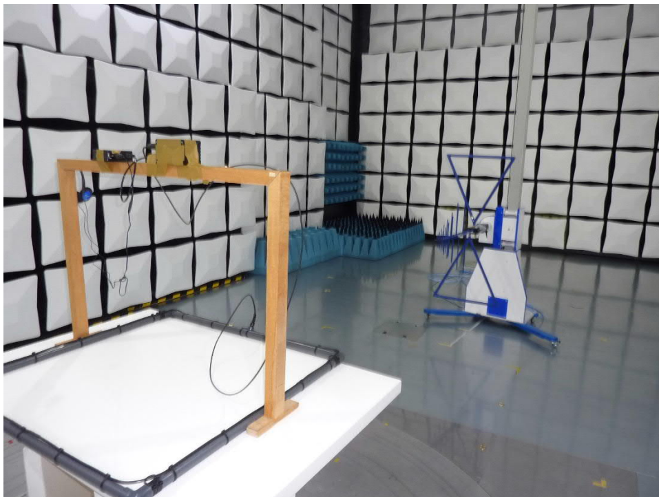
201626_08: EUT setup radiated emission 1 x 1 m frame coil below 1 GHz
