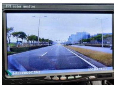
Figure 13: Make sure the skyline is in the center of the screen or in web-app
