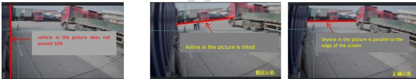
Figure 15: Installation requirements, wrong for the middle and correct for the right figure
