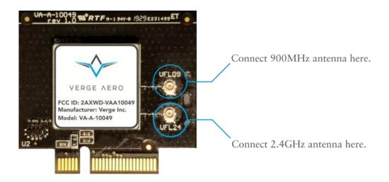
The VA-A-10049 module is authorized for use with a 900MHz antenna with a stated gain of up to 8dBi, and a 2.4GHz antenna with a stated gain of up to 14dBi. System integrators are responsible for ensuring that the gain of the selected antenna, in all directions, does not exceed those limits.
