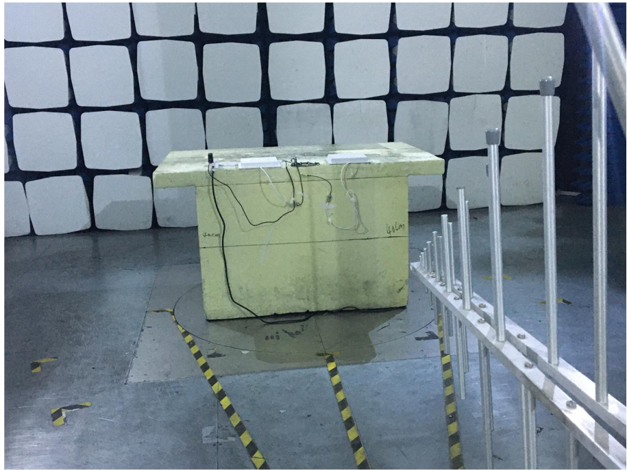
Radiation Emission Test Setup (30MHz to 1GHz)
