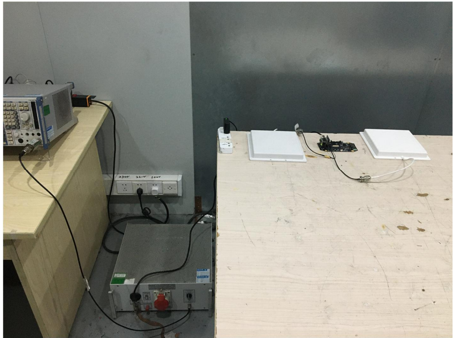
Conducted Emission Test Setup
