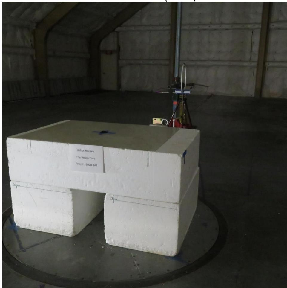
EUT set up in OATS, 9kHz – 30MHz, front
