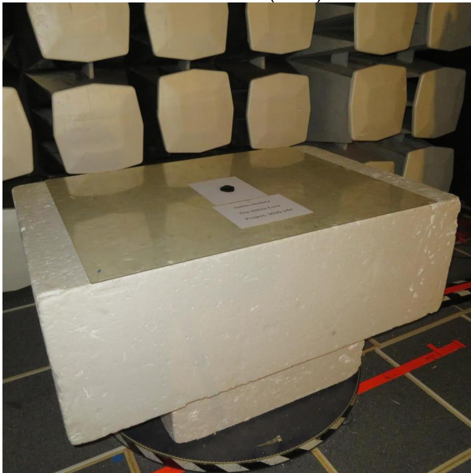
EUT set up in chamber, prescans
