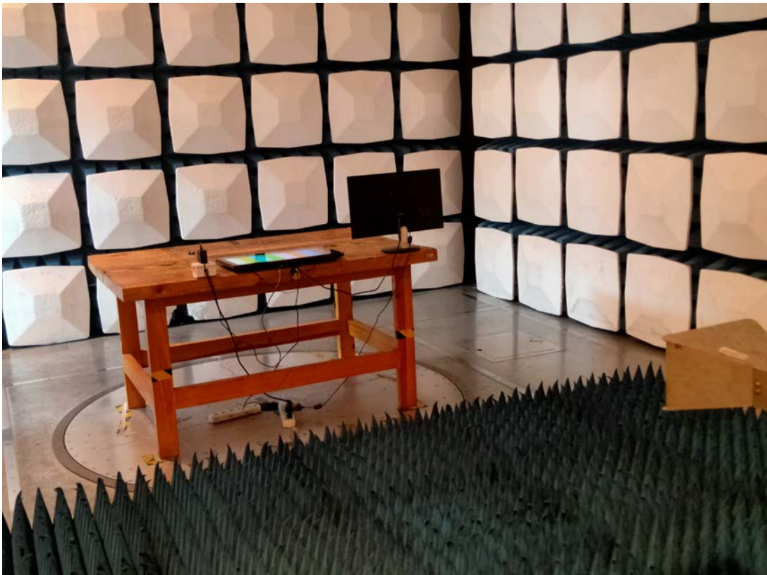
Radiated Emission Above 1GHz Rear View- TAV-21
