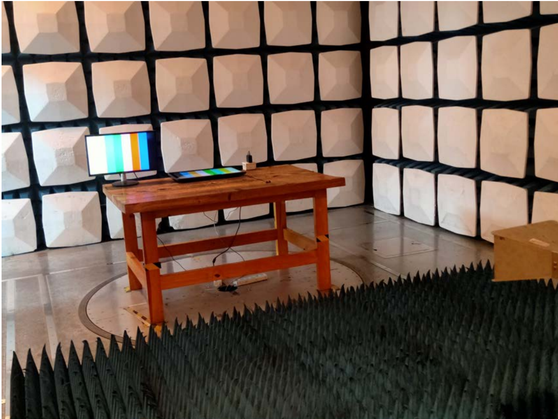
Radiated Emission Above 1GHz Rear View- TAV-21
