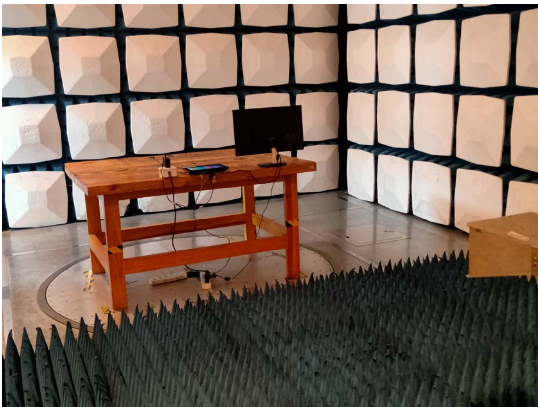
Radiated Emission Above 1GHz Rear View- TAV-10
